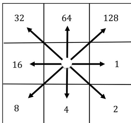
Figure 2. Flow direction in the 8 flow direction model (1 - East; 2 - South East; 4 - South; 8 - South West; 16 - West; 32 - North West; 64 - North; 128 - North East).
