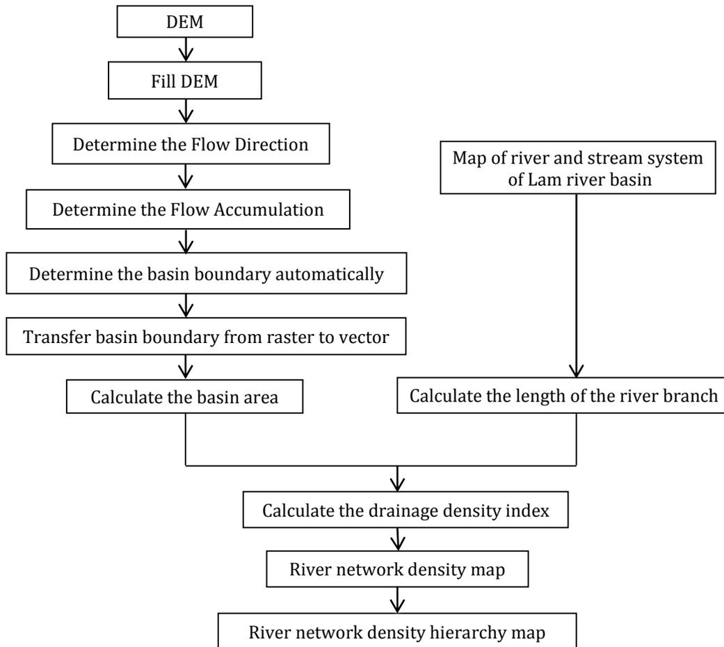
Figure 1. The process of establishing a drainage density hierarchy map.
