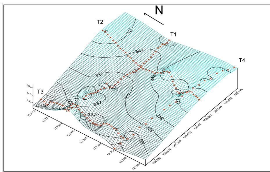
Figure 9. Iso - depth diagram of the top of the bedrock of La Nga formation.
