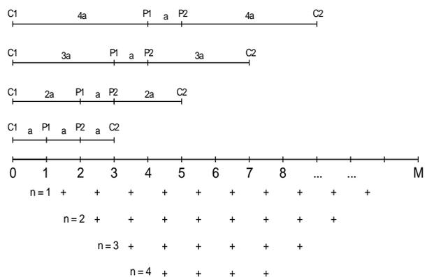
Hinh 3. Arrangement of data points in the pseudosection for the W - S array with  $n$  varying from 1 to 4.
