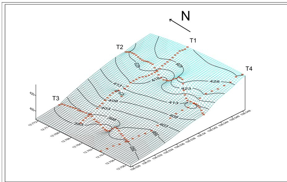
Figure 8. Iso - depth diagram of the top of basalt layer.
