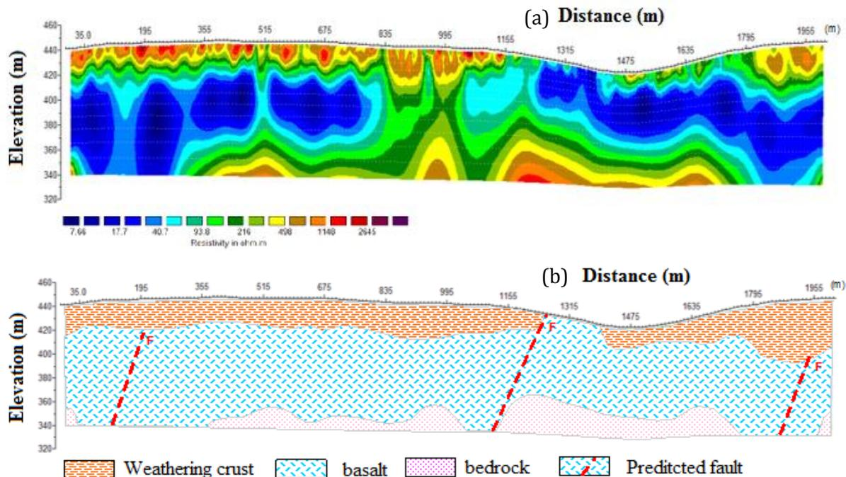
Figure 6. The 2D resistivity imaging result on profile T2: inversed resistivity cross section (a) and geo - electrical cross - section (b).
