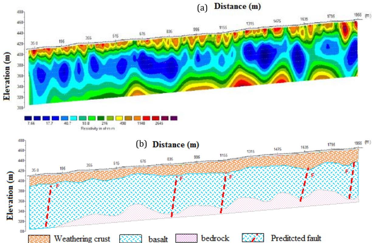
Figure 5. The 2D resistivity imaging result on profile T1: inversed resistivity cross - section (a) and geo - electrical cross - section (b).
