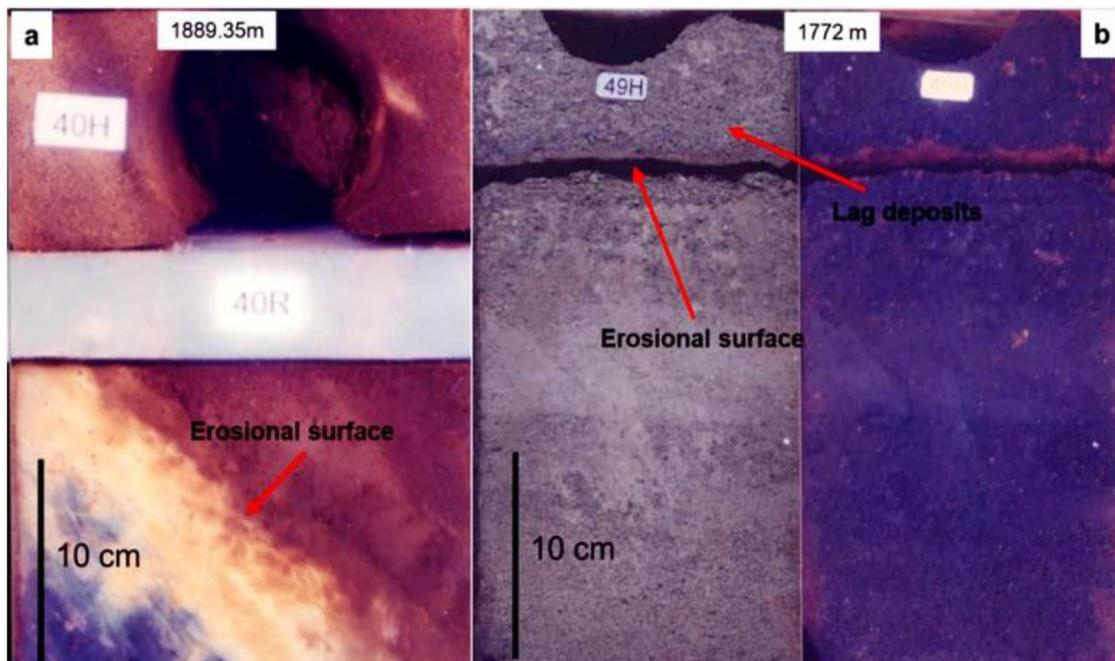
Figure 2 Core pictures show erosional surfaces/channel bases and lag deposits (thin bed of sands having coarser grain size occurring at bases of channels), a. The channel base in well 2, b. The channel base and lag deposits in well 3.
