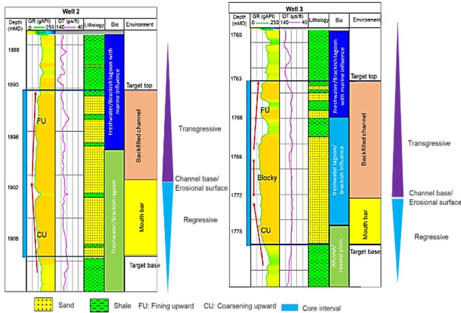
Figure 6. Depositional environment of well 2 (left) and well 3 (right). The coarsening upward succession in the both two wells was interpreted as mouth bar deposits formed during regressive phase. The blocky succession (well 2) and the blocky to fining upward succession (well 3) were interpreted as backfilled distributary channel deposits formed during transgressive phase.
