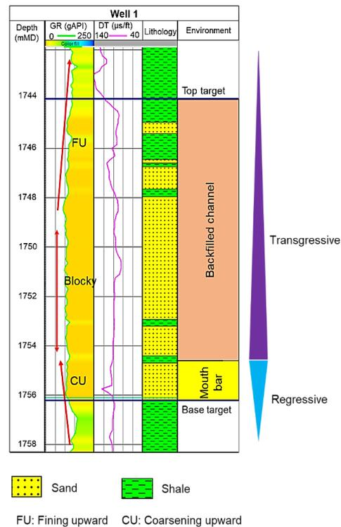
Figure 7. Depositional environment of well 1. The coarsening upward succession was interpreted as mouth bar deposits formed during regressive phase. The blocky to fining upward succession was interpreted as backfilled distributary channel deposits formed during transgressive phase.
