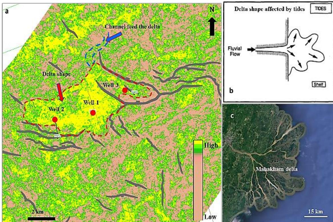
Figure 8. A deltaic shape, a. The result of similarity of the relative acoustic impedance attribute indicating high similarity of the relative acoustic impedance at the well locations, which shows a deltaic shape. This shape indicated that the delta could be slightly affected by tides, b. schematic of a delta shape affected by tides, c. Mahakham delta.
