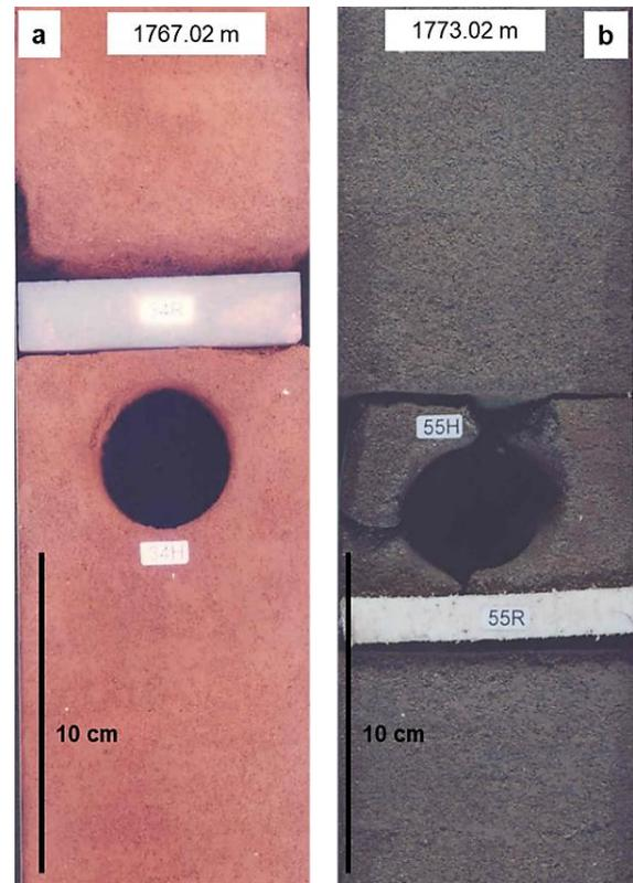
Figure 3. Core pictures show massive sands in well 3, a. Massive sands above the erosional surface, b. Massive sands below the erosional surface.
