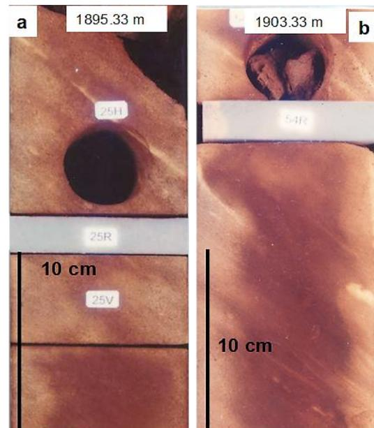
Figure 4. Core pictures show Parallel laminated sands in well 2, a. Parallel laminated sands above the erosional surface, b. Parallel laminated sands below the erosional surface.
