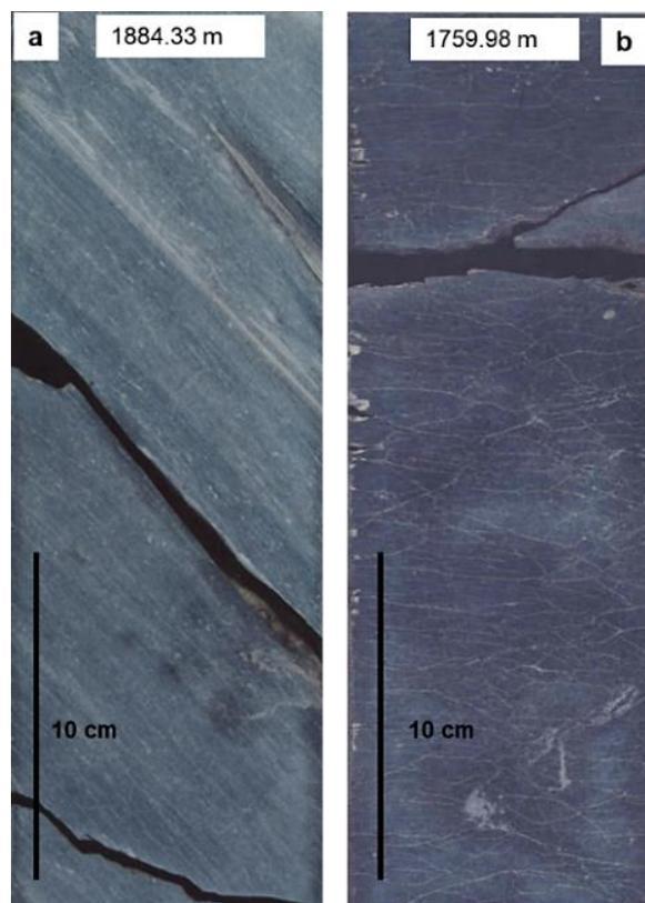
Figure 5. Core pictures show parallel laminated and laminated silty clay in well 2 and well 3, a. Parallel laminated silty clay in well 2, b. Laminated silty clay in well 3. The parallel laminated and laminated silty clay indicate a low energy environment.
