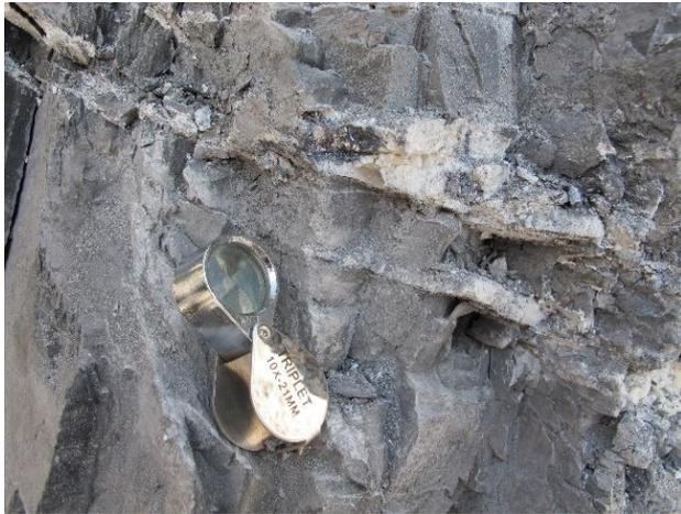
Figure 2. Sulphides disseminated in broken quartz vein and in clay schist of Dong Bua copper mine.
