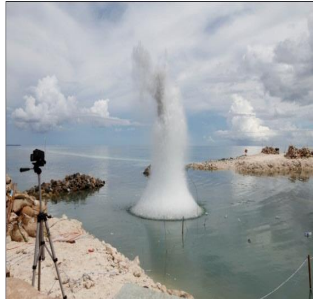
Figure 3. The underwater explosion in Son Ca island in 2013 (600g TNT charge) (Vu, 2014)
