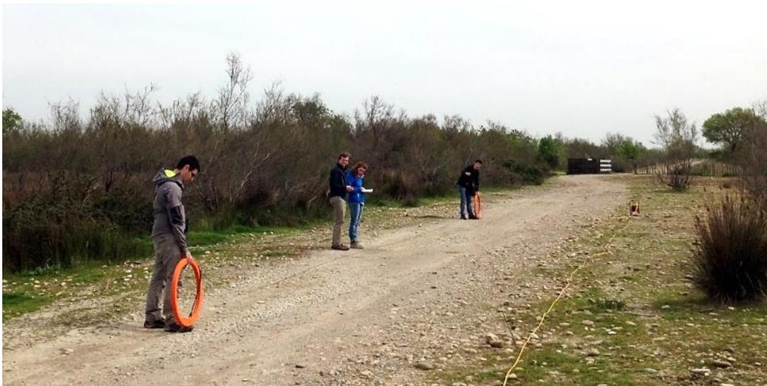
Figure 6. EM34 measurement in study area.
