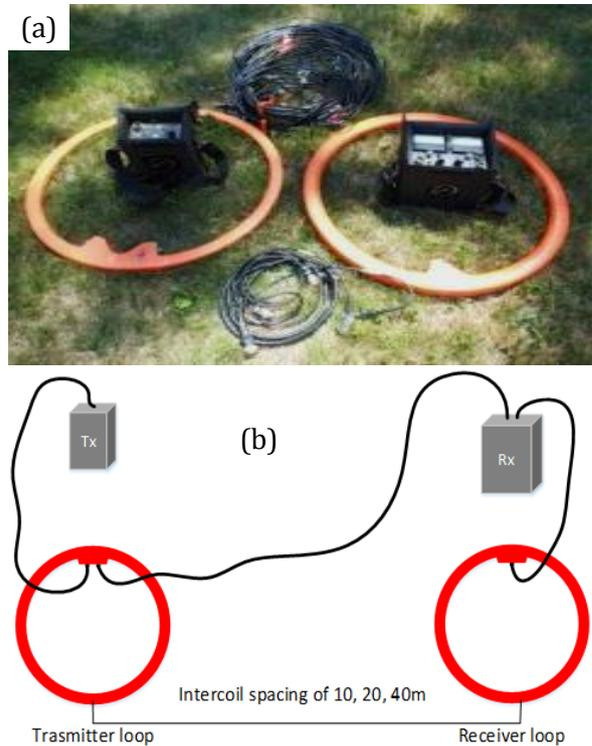
Figure 1. Geonics Electromagnetic EM34-3 instrument applied in study area.
