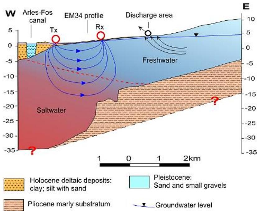
Figure 7. Principle of EM34 profile with regard to interface between fresh and salt water of cross section I-I'.
