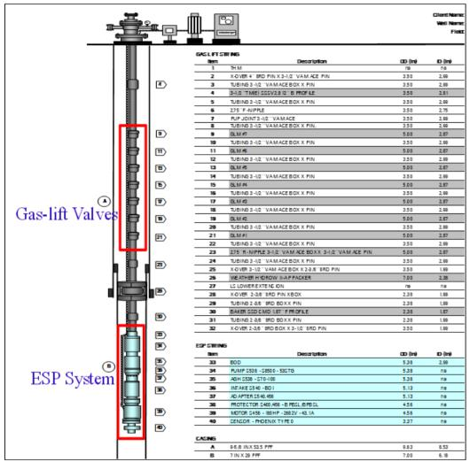
Figure 4. ESP and GL combination system schematic.
