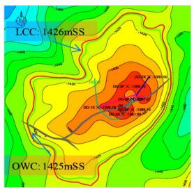
Figure 1. Area of BII.2.20 heavy oil reservoir with well locations (Lamson JOC, 2016).
