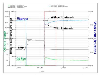
Figure 7. Simulation results of diesel injection application for ESP well.
