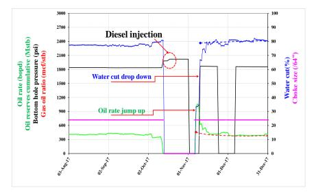
Figure 8. Diesel injection solution applied for ESP wells in Dong Do heavy oil field.
