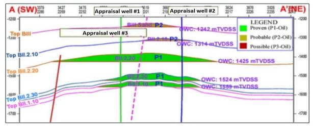
Figure 2. Dong Do heavy oil field cross-section with oil-water contacts (Lamson JOC, 2016).
