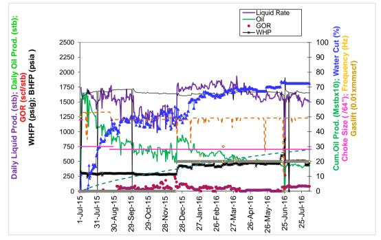
Figure 6. Well production performance with ESP & gaslift combination.
