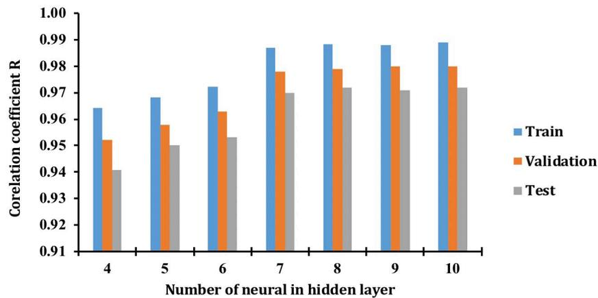
Figure 3. Results of correlation coefficient with different number of neural in the hidden layer.
