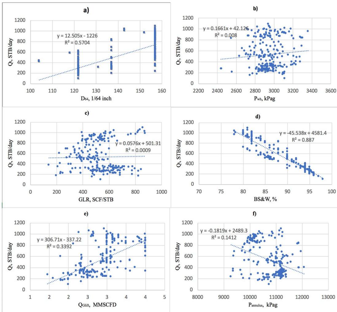
Figure 1. Correlations between production flow rate ( $Q_1$ ) and a) choke size; b) wellhead pressure ( $P_{wh}$ ); c) ratio of gas to liquid (GLR); d) Free water, sediment and emulsion (BS&W); e) injected gas lift rate  $Q_{glift}$ ; f) injected gas lift pressure ( $P_{annulus}$ ).
